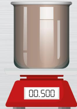
Fill the container with un-frozen liquid mix right to the brim and place on the scales. Make a note of the weight of the mixture.
