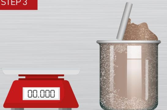
Clean and dry the container. Fill the container with frozen product directly from the machine; with a straight edge, level the top off.
