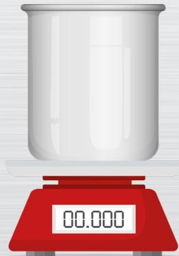
Place an empty container on a set of scales and zero the reading.
